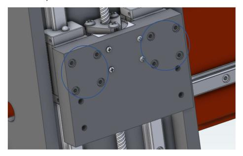
3. Square the Z bearing block to the bed of the machine using a carpenter's or machinist's square
