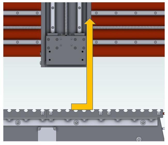
4. While holding the bearing block square, re-tighten the 8 m4 x 18 bolts.
