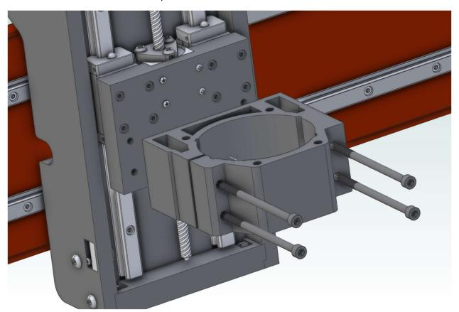
2. Loosen the 8 m4x18 bolts (it is recommended to use a hand tool for this to avoid stripping the bolts). Do not remove the bolts.
