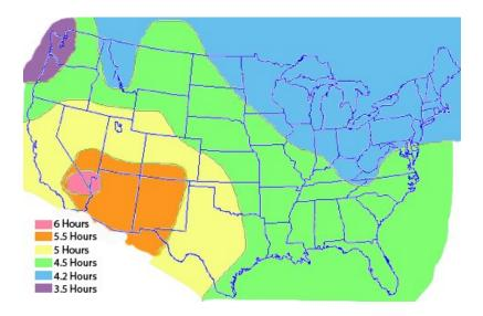
Divide this into the watt-hours needed to determine the size of solar cell you'll need. For instance, if you live in an area that averages 4 hours per day, you'll need a 144 watt-hour / 4 hours = 36 watt solar cell.
