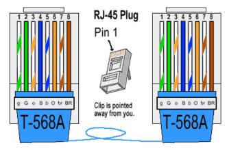
The AyrMesh Hub can accept voltages from 9 to 18 Volts DC – the positive voltage is on lines 4 and 5, and the negative (ground) is on lines 7 and 8. If you are handy with electrical connections, this is the easiest way to power the Hub.
